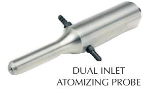
With the wide dispersion atomizing probe, the liquid which is dispensed onto the probe surface via a small tube runs downward and spreads out as a thin film on the tip surface. The oscillations disintegrate the liquid into micro-droplets, and eject them to produce a fine, low velocity spray.
